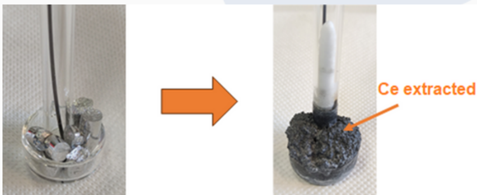
Figure 7: Experimental assembly used for the reductive extraction experiments of cerium on a metallic alloy.
